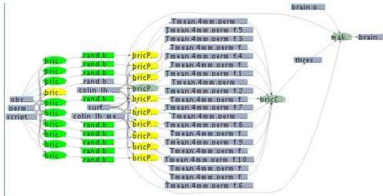
**Figure 2.** The execution of a small subset of the aphasia study analysis workflow. The colors of the boxes indicate if the task has completed (green) or is executing (yellow). Lines represent data dependencies.
