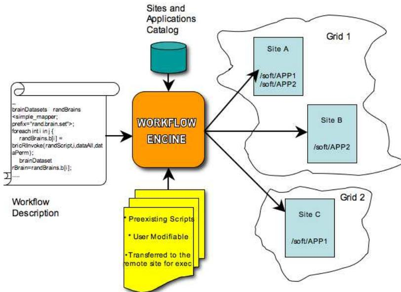
**Figure 1.** The components of a workflow based application
