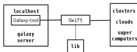
**Figure 1: Swift acting as an interface between locally installed Galaxy tools and remotely located resources.**
