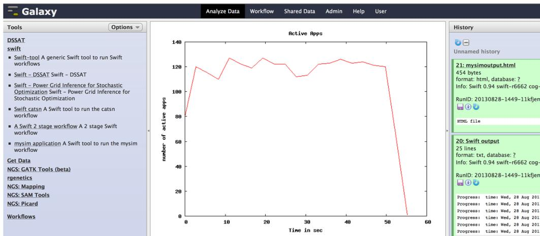
Figure 6: Screen capture of a post execution view of a Swift tool. The plot shows the number of parallel active jobs during the run of a 2000-task application.
