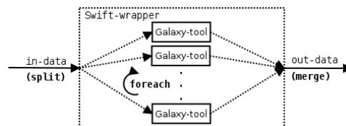
Figure 4: Swift wrapper to Galaxy tool. Input data from the Galaxy tool input is split, the base tool is run under a Swift foreach on each fragment, and the results are merged and presented as the Galaxy tool output.
